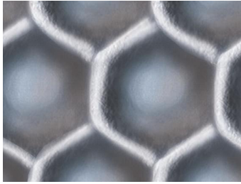
Picture 6: CELLS OF ANILOX ROLL, ENGRAVED WITH ULTRA MELT™ TECHNOLOGY
