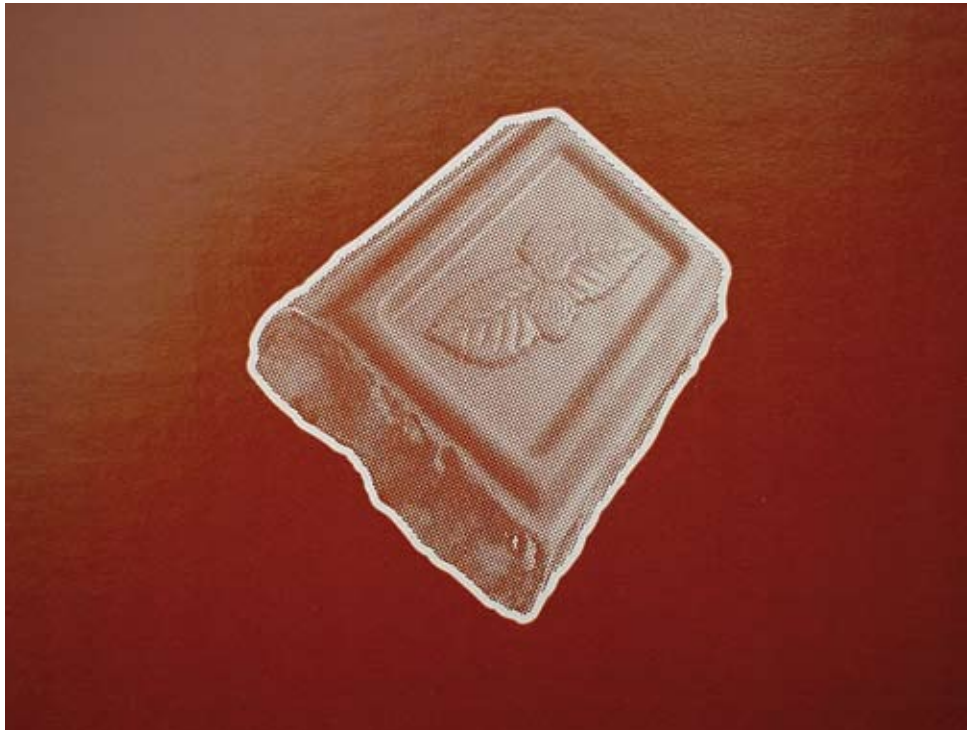
B-flute, white coated Full tone and 26 l/cm screen on one printing plate
